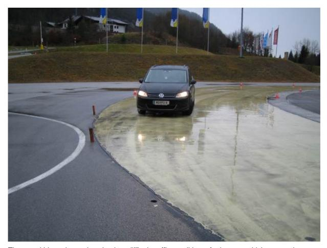
The wet skid pan is used to simulate difficult traffic conditions, for instance driving on an icy road. This calls for a special coating of the road surface, which has been created in the Driving Centre in Saalfelden by the use of the PUR coating PCI Apoten PU.
